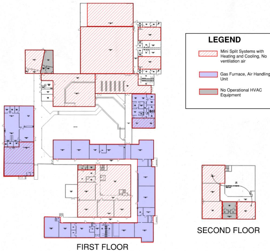
Figure 1 HVAC system type map
